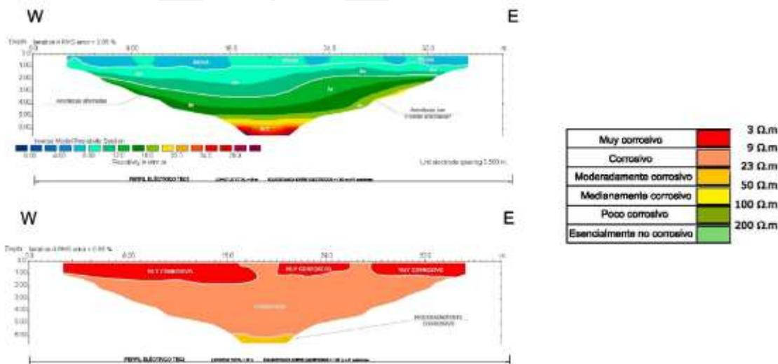
Fig. 5: Electrical Tomography sections. Up: with geological interpretation. Down: with corrosion potential
